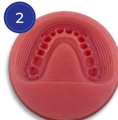
Puck is custom milled to create patient-specific tooth sockets
