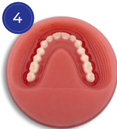
Custom dentin layer is milled
