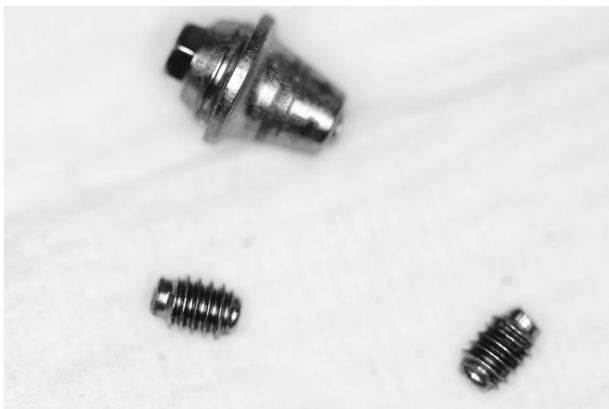
Figure 2 Retrieved fractured components of the anterior multiunit abutments.
