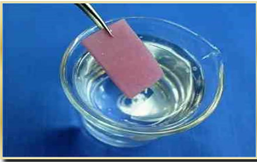
**Figure 1.** Chemical polishing of acrylic resin specimen immersed in methyl-methacrylate monomer
