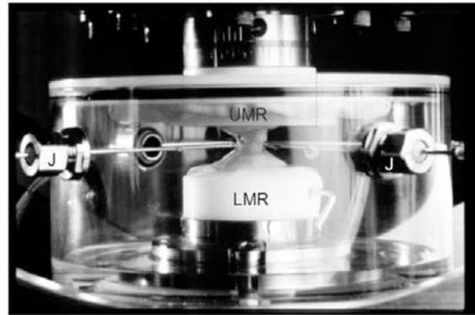
**Figure 1:** ART 1 Environmental Chamber. LMR – lower mounting ring. UMR – upper mounting ring (ring is outlined by the dashed line). The UMR is fixed to the load cell, which is just visible at the top of the image, and does not move. The LMR moves laterally and vertically to produce the chewing motion. J – Lubricating jets. Four adjustable jets spaced uniformly around the sample direct the lubricating media onto the samples.
