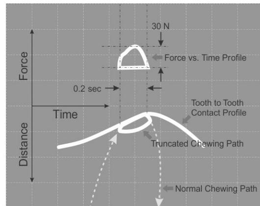
**Figure 2:** Cathode Ray Display of ART 1. Two profiles are displayed: force vs. time (upper profile) and distance vs. time (lower profile). The contact curve is generated by moving the lower tooth laterally against the upper tooth under a constant force.
