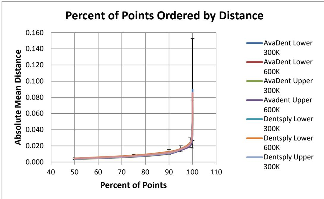
**Figure 7:** Quality of alignment of digital model. All alignments are to the baseline model. The error bars are the largest standard deviation of the eight comparisons for a given percentage.
