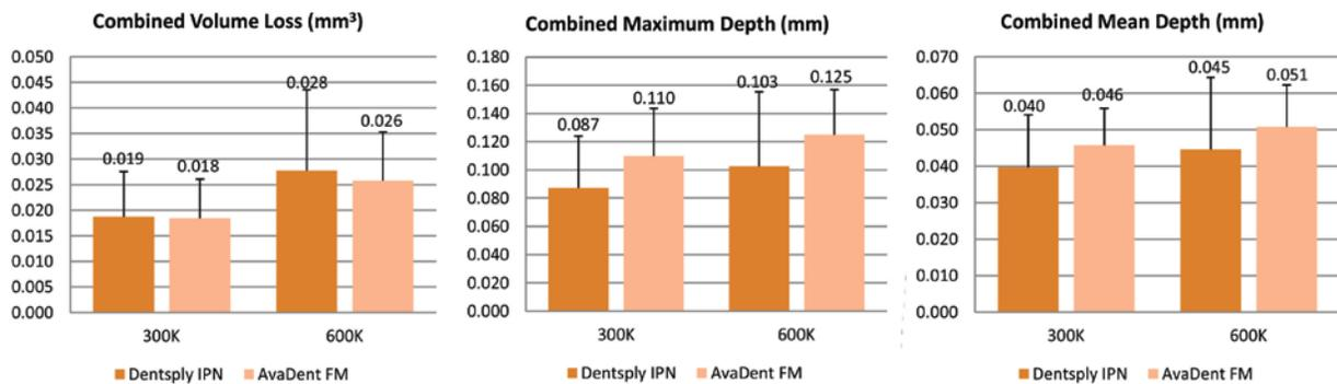
**Figure 6: Combined Wear Results.** Upper and lower values for a wear parameter were combined to give the total wear for the two materials. There were no statistical differences between Dentsply IPN and AvaDent FM. The number of samples for Dentsply IPN and AvaDent FM were 4 and 5, respectively. The error bars represent one standard deviation.
