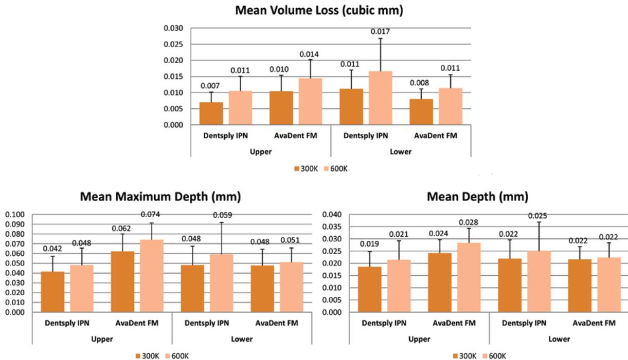
**Figure 5: Average Parameter Values.** There were no statistical differences between Dentsply IPN and AvaDent FM. The number of samples for Dentsply IPN and AvaDent FM were 4 and 5, respectively. The error bars represent one standard deviation.
