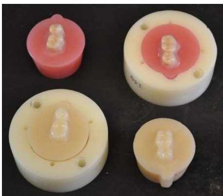
Figure 3a: Test samples with mounting rings AvaDent FM samples have a white base; Ivoclar DCL samples have a pink base.
