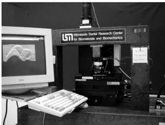
Figure 4: MDRCBB Contact Profiling System. This system uses a unique method to profile surfaces. The stylus is mounted on an extensometer, which is very sensitive to vertical movement. The stylus is brought into contact with the surface and deflected upwards a fixed amount. As the surface moves under the stylus horizontally, the stylus wants to move up or down depending on the anatomy of the surface. Closed loop circuitry moves the surface in the direction opposite to the deflection of the stylus; thus, keeping the stylus tip at the fixed offset. The vertical movement of the stylus and the surface are combined to determine the height of the surface. The final shape of the surface is corrected for the shape of the stylus tip.
