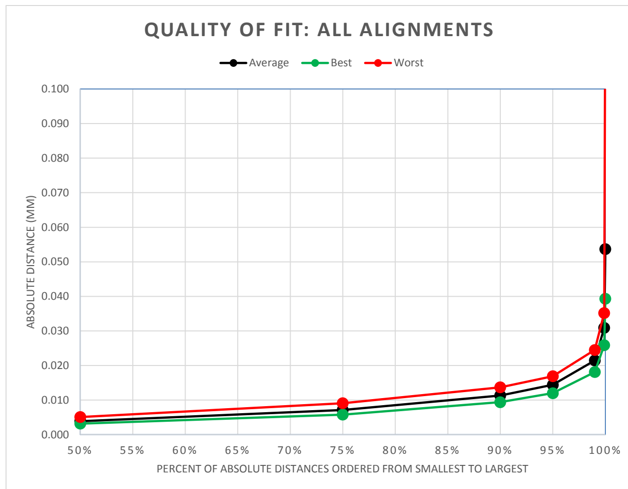
Figure 14: Quality of alignment of digital model. All alignments are to the baseline model. Results are the average of all samples (Ivoclar DCL Lower, Ivoclar DCL Upper, AvaDent Lower, Avadent Upper). The black line is the average, the red line is the upper limit, and the green line is the lower limit.
